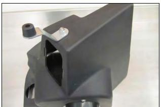
7. Turn the Cold Air Box upside down and mount the Bottom Bracket (#26) using one 1/4-20x3/4" Hex Head Bolt (#11), 1/4" Flat Washer (#12), and 1/4"Lock Nut (#14) as shown. Next using one 8-32x5/8" Button Head Screw (#18), and the #8 Kep Nut (#19), attach the Plastic Bumper (#20) to the Backet as shown.
