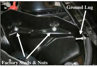
**11.** Install the Airaid CAB assembly into the vehicle locating the factory grommets over the factory studs. Reinstall the factory nuts from step **2.** onto the studs. Reinstall the factory ground lug thru the CAB and into the side bracket using one flat washer (#12), and one 6mm flange nut (#16).
