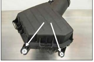
**5.** Remove the two steel inserts, and grommets from the factory airbox. Save these pieces, they will be reused.
