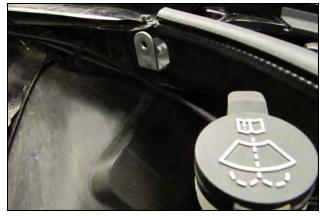
**10.** Replace the ground lug from step #11 with the Side Bracket (#25) as shown using one 6mmx12mm Hex Head Bolt (#14), and Lock Washer (#12).
