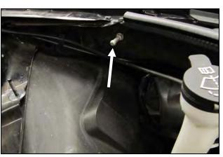
**9.** Using a 10mm wrench, remove and save the ground lug from the driver's side inner fender. It will be reused in step #11.
