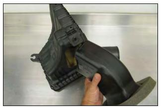
**4.** Compress the sides of the factory intake scoop and remove it from the factory airbox. It will be reused in step #8.
