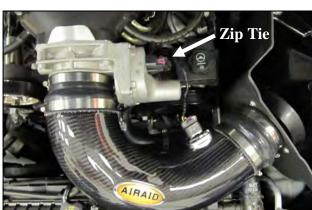
**14.** Install the Airaid Intake Tube into the Hump Hose first, and then into the Reducing Coupler. Adjust for fit, and tighten all four hose clamps. Re connect the Mass Airflow Sensor and secure the wire harness to the throt-tlebody harness using a single Zip Tie (#27)
