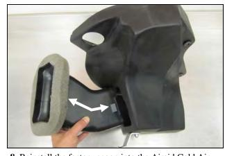
**8.** Reinstall the factory scoop into the Airaid Cold Air Box with the inlet angled upward . It will snap into
