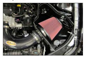
**16.** Install the Airaid Premium Filter (#1) onto the Filter Adapter and tighten the Clamp. Next install the Weather Strip (#8) onto the top of the Cold Air Box with the contour rolling away from the Filter.
