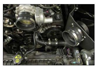
**12.** Install the Hump Hose (#6) onto the Filter Adapter using two #64 hose clamps (#23). Next install the Reducing Coupler (#5) with one #60 Hose Clamp (#22) on the throttlebody side and one #68 Hose Clamp (#24) on the open end.
