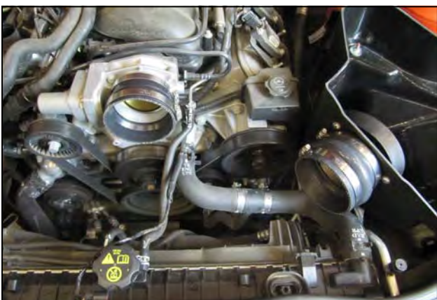
15. Install the Hump Hose (#4) onto the Filter Adapter using two #64 Hose Clamps (#24). Next install the Reducing Coupler (#6) with one #60 Hose Clamp (#23) on the throttlebody and one #68 Hose Clamp (#25) on the open end.
