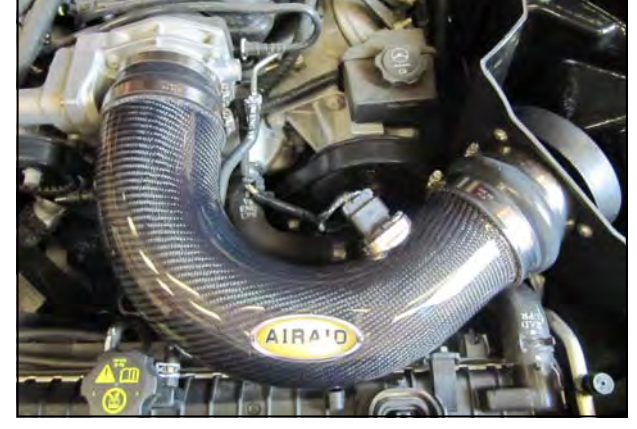
17. Install the Airaid Intake Tube (#2) into the Hump Hose first, and then into the reducing coupler. Adjust for fit, and tighten all four Hose Camps. It is Very important to verify that the Intake Tube is not rubbing on the Radiator or the hood.
