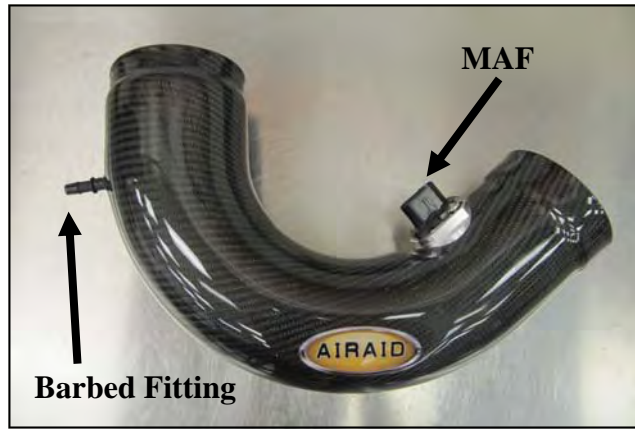
16. Transfer the Mass Air Flow sensor into the Airaid Intake Tube (#2) and secure it using two 8-32x3/8" Button Head Screws (#22). Do not attempt to reuse the factory screws. Install the Barbed Fitting (#9) and Grommet (#10) into the 5/8" hole in the Tube.
