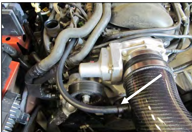
18. Install the 3/8"x18" breather hose between the Barbed Fitting and the steel crankcase breather tube on the valve cover. Refer to step #2. Install the Speed Clamp (#11) over the Breather Hose at the Barbed Fitting as shown.
