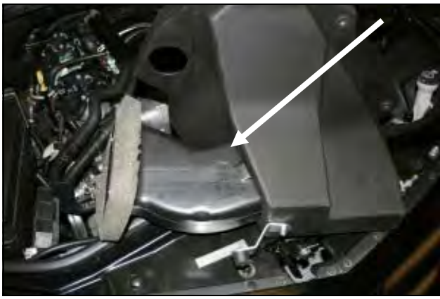
10. Reinstall the factory scoop into the Airaid CAB. It will snap into place.
