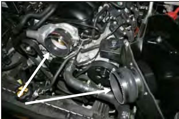
14. Install the hump hose (#6) onto the filter adapter using two #64 hose clamps (#23). Next install the reducing coupler (#5) with one #60 hose clamp (#22) on the throttlebody and one #68 hose clamp (#24) on the large end.
