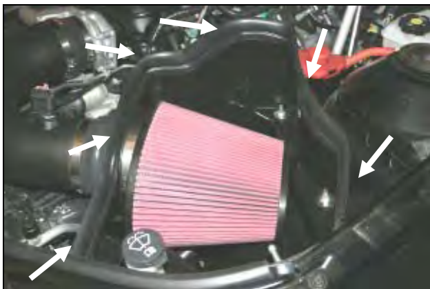
17. Install the Airaid Premium Filter (#1) onto the filter adapter and tighten the clamp. Next install the weather strip onto the top of the CAB. For ease of installation, start the front of the CAB near the radiator and work your way around towards the fender. Reinstall the engine beauty cover and oil fill cap.
