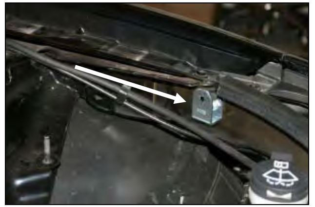
12. Replace the ground lug from step #11 with the side bracket (#25) as shown using one 6mmx12mm hex bolt (#14), and lock washer (#12).
