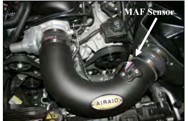
15. Install the Airaid Intake Tube (#2) into the hump hose first, and then into the reducing coupler. Adjust for fit, and tighten all four hose clamps. Next install the MAF sensor into the tube and secure it using two 8-32x3/8" button head screws (#16).
