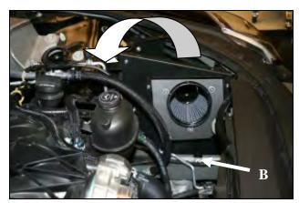
**13. A)** Lower the Airaid Performance Air box assembly into the engine cavity. Insert the Well Nut into the Factory core support grommet and rotate the assembly rearward until the bracket rests on the shock tower and the MAF panel's lower tab hole is lined up with the Tapped Chassis bolt hole from step **5. B)** Secure the assembly by using the 1/4-20x 3/4 Bolt(#19).
