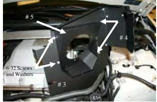
**6.** Install the Adapter Panel (#5) to the MAF Panel (#3) as shown using four 6-32 screws (#12), 6-32 Kep nuts, and #6 flat washers (#14). Attach the Rear Panel (#4) to the MAF Panel using two 6-32 screws.
