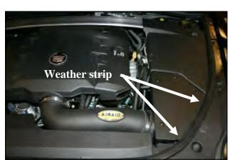
**16. A)** Install the 11" Weather Strip (#11) onto the curved edge of the top cover (#6) and install the top cover onto the Airaid filter box using the four 1/4-20 Black screws.(#22). **B)** Line up the intake bracket with the fender bolt hole, and secure the assembly using the factory bolt. Reinstall the Factory engine and shock tower covers .Note: These steps must be performed in order to avoid difficulty with bolt hole alignment.
