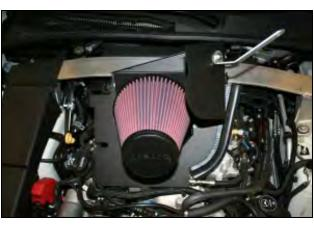
**12.** Install the Bracket (#28) on to the Rear Panel (#3) as shown using one 1/4-20 Button Head Screw (#17), 1/4" Flat Washer (#20), and 1/4" Serrated Nut(#21). Complete the assembly by attaching the Airaid Premium Filter (#1) to the Filter Adapter (#10).
