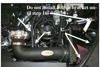
**15. A)** Replace the factory breather line on the valve cover with the 26" Airaid Breather Hose(#12). **B)** Secure the breather hose to the intake tube nipple using the black Speed Clamp (#32). **C)** Slide the Edge Clip Cable Ties (#31) about 6" apart along the fender pinch weld and return the coolant line to it's original location. Secure the coolant line using the cable ties and trim off excess.
