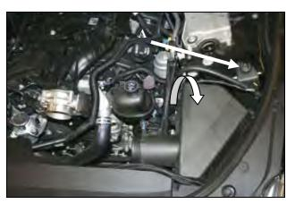
**3. A**) Remove the factory fender bolt securing the air box assembly. Next pull out the coolant line from atop the air box lid and gently rotate the air box assembly towards the front of the vehicle. The air box assembly is now free and should be removed from vehicle.
