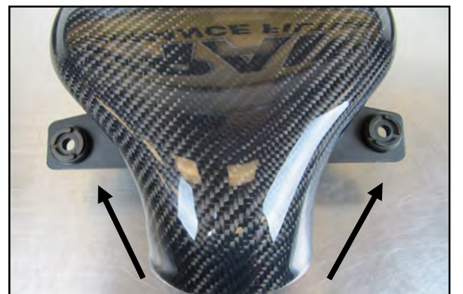
9. Transfer the factory intake tube mounting grommets into the Tube Brackets as shown.
