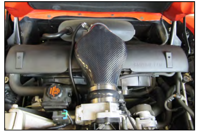
15. Check the alignment of all the intake components and adjust if necessary. Begin tightening the clamps from the front of the intake and move back towards the throttle body. Reconnect the battery.
