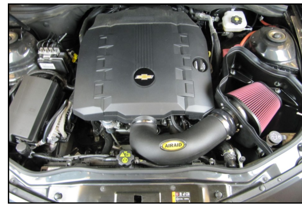
18. Double check your work! Make sure there is no foreign material in the intake path. Make sure all clamps, hoses, bolts, and screws are tight. Double check the hood clearance! Reconnect the negative battery cable.
