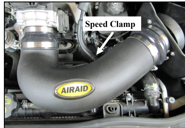
15. Install the Airaid Intake Tube into the hump hose first, and then into the coupler. Adjust for fit, and tighten all four Hose Clamps. Reconnect the PCV breather using the supplied PCV Hose. Slide the hose onto the factory hard line and onto the Intake Tube's Barbed Fitting. Use the Speed Clamp (#13) to secure the Hose onto the Fitting. Reconnect the Mass Air Flow meter.
