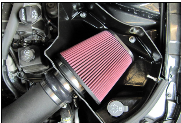
16. Install the Airaid Premium Filter onto the Filter Adapter and tighten the clamp.
