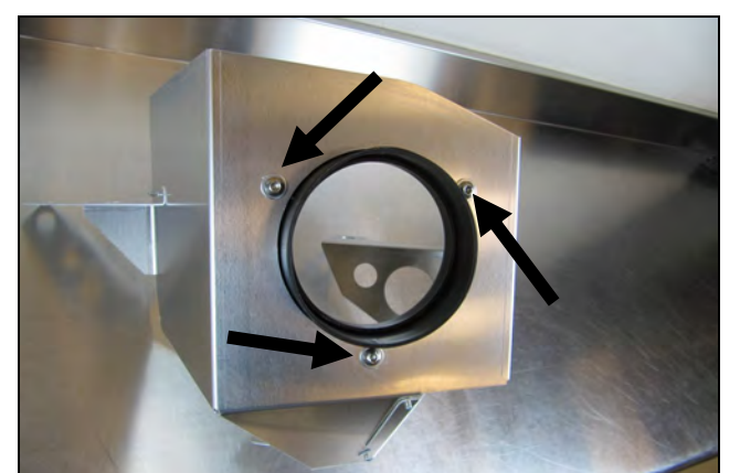
6. Install the Filter Adapter onto the Air Dam as shown using the three Button Head Screws and Flat washers.
