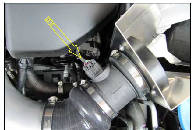
18. Reconnect the Air Flow Meter and reinstall the Positive terminal cover removed in step 1.
