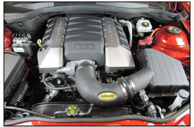
12. Reinstall the engine cover and oil cap. Reconnect the battery terminal.
