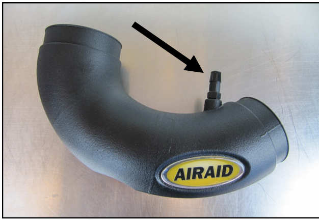
10. Install the Barbed Fitting into the Airaid Intake tube as shown.
