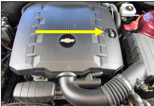
1. Disconnect the negative battery terminal. Remove the oil cap and lift up on the engine cover to unseat it from the mounting grommet. Replace the oil cap for now to prevent debris from entering the valve cover.
