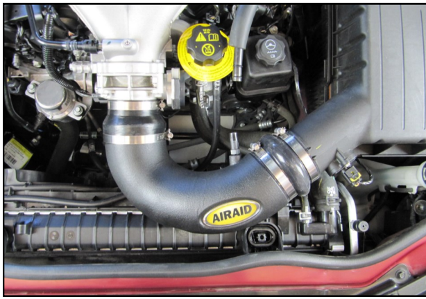
11. Insert the Intake Tube assembly into the Hump Hose first then into the Coupler on the throttle body. Align the components and tighten the Clamps.
