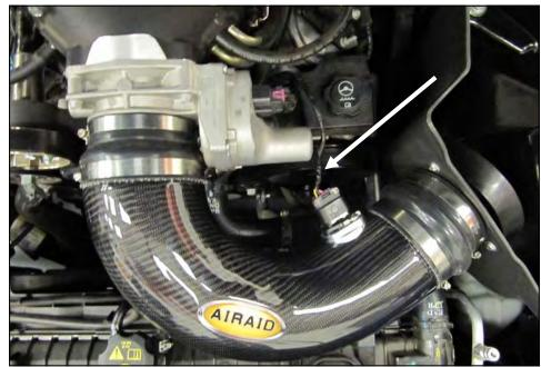
5. Install the 3/8" Breather Hose onto the Barbed Fitting and carefully route it behind the pulleys following the wiring harness. Connect the other end of the breather line to the hard line from step 1. Secure the breather line behind using the two remaining Zip Ties once you have determined it is safe from all moving parts
