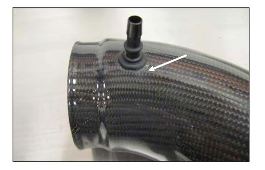
**3.** Install the 3/8" Grommet and the Barbed Fitting into the small hole in the Intake Tube as shown.
