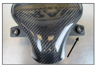
**3.** Transfer the factory intake tube mounting grommets into the Tube Brackets as shown.
