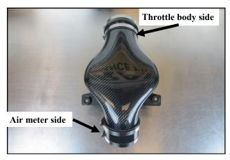
**4.** Slide the Hump Hose and #64 clamps onto the throttle body side of the Intake Tube and the Coupler and #56 Clamps onto the air meter side. Leave all clamps loose at this time.
