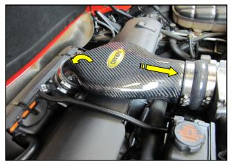
**5**. Install the Airaid Tube assembly onto the throttle body and lower it downward towards the Mass Air Flow meter.
