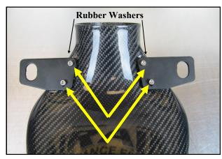
**2.** Set the Rubber Washers (#8) onto the Intake Tube and align with the threaded holes of the inserts.
