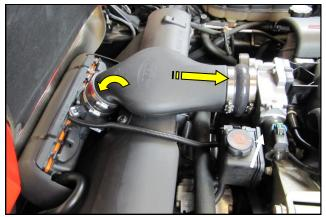
**5**. Install the Airaid Tube assembly onto the throttle body and lower it downward towards the Mass Air Flow meter.
