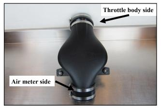
**4.** Slide the Hump Hose and #64 clamps onto the throttle body side of the Intake Tube and the Coupler and #56 Clamps onto the air meter side. Leave all clamps loose at this time.
