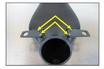
**2.** Install the Tube Brackets onto the Intake Tube as shown using the 8-32 Socket Head Screws (# 4)
