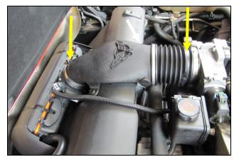
1. <u>Disconnect the negative battery cable!</u> Loosen the intake tube clamps on the throttle body and the Mass Air Flow meter. Unseat the intake tube mounting grommets from the posts on the radiator shroud and remove the factory intake tube.
