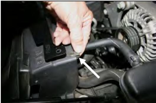
**13.** Slide one clip nut (#10) over the outside end of the plastic radiator cover and align it with the hole in the air dam. Install one rubber washer (#11) over the threads of the clip nut, and then align the air dam hole over the washer. Add one more rubber washer, one #8 flat washer (#9), and one 8-32x1/4" button head bolt (#8) to secure the air dam. Repeat this step on the passenger side. Refer to the line drawing on page one.
