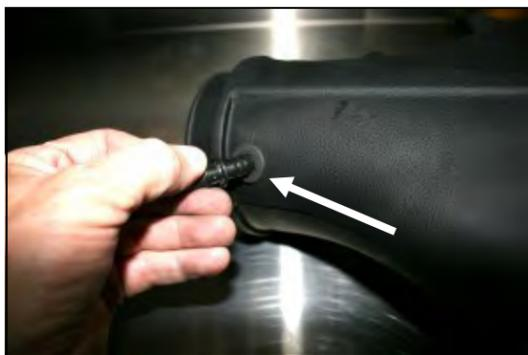
**7. Install the provided grommet (#13) into the hole in the Airaid Intake Tube (#2). Next install the factory plastic breather fitting removed in step #6 into the grommet.**
