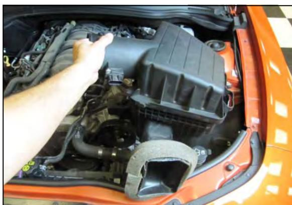
5. Lift the complete air box assembly straight up, and out of the vehicle.
