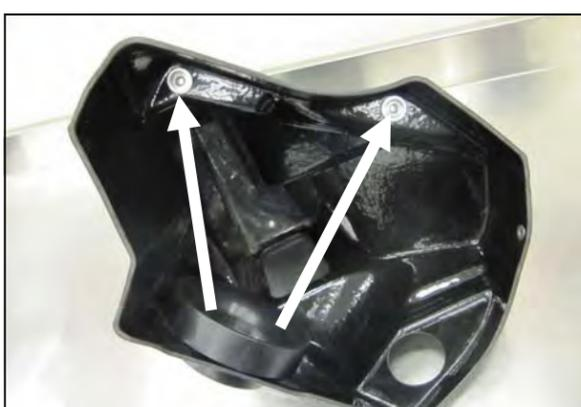
8. Transfer the factory grommets and inserts into the Cold Air Box.
