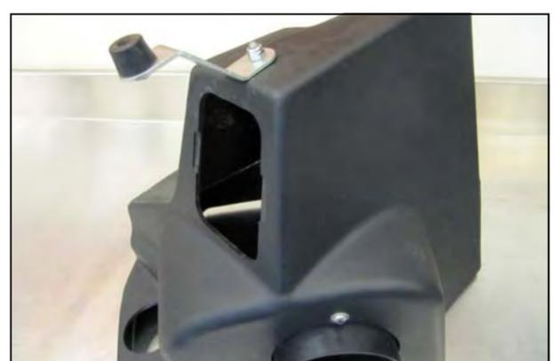
9. Turn the CAB upside down and mount the Lower Bracket (#20) to the bottom using the 1/4-20 x 3/4" Hex Bolt (#17), 1/4" Flat Washer (#16), and 1/4" Nylock Nut (#18) as shown. Next- using the 8-32x5/8" Button Head Screw (#19), and the #8 Kep Nut (#19), attach the plastic Bumper (#12) to the Bracket as shown.
