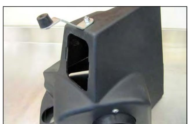
7. Remove the factory airbox grommets and the steel inserts inside of them.
