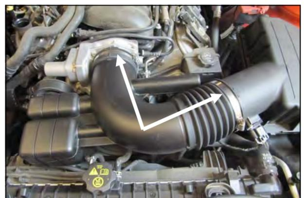
3. Loosen the clamps on the throttlebody and the airbox and remove the intake tube from the vehicle.
