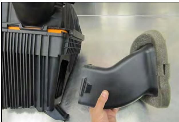
10. Compress the sides of the factory intake scoop and remove it from the airbox.
