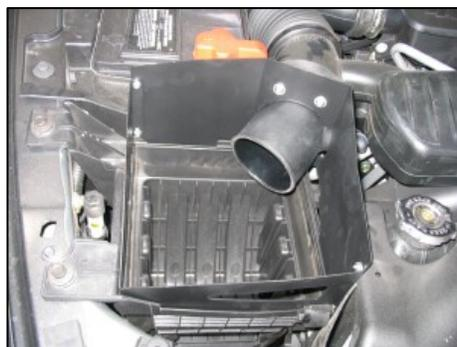
6. Install the Airaid Cool Air Dam assembly on top of the factory air filter base. Tighten hose clamp.
