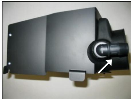
5. Install the supplied nylon fitting into the air filter adaptor as shown.
