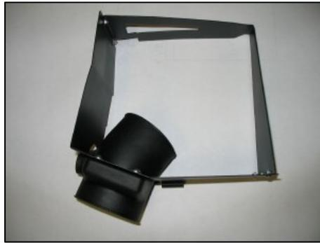
4. Using the supplied #6 screws, nuts and washers, assemble the two panels as shown above. Next, install the supplied sir filter adapter using the supplied 1/4-20 bolts and washers.
