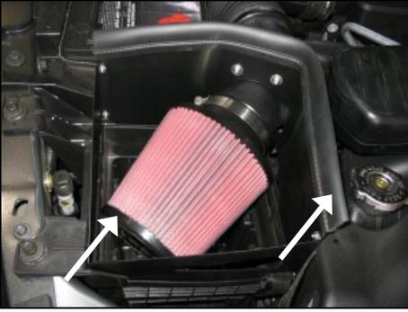
9. Install the Airaid Premium Filter on the end of the air filter adaptor. Install the supplied weather strip on the Cool Air Dam. (*Note: start from one end and work your way around to insure proper alignment of weather strip.*)
