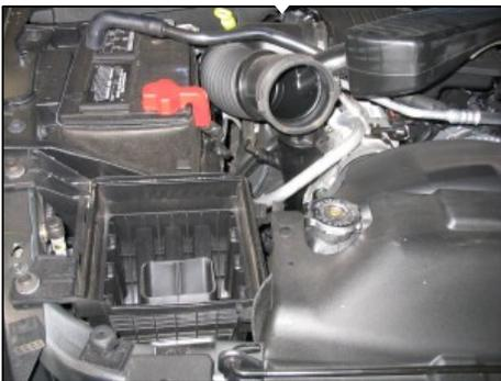
2. Loosen hose clamp on air box lid and remove lid from air box base.
