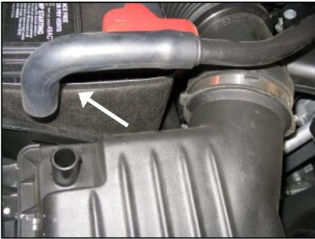
1. Disconnect negative battery cable. Disconnect the factory breather hose and remove from the vehicle. (*Note: 4.7L engines require the removal of the breather hose end section only. 5.7L Hemi required removal of entire hose assembly.*)
