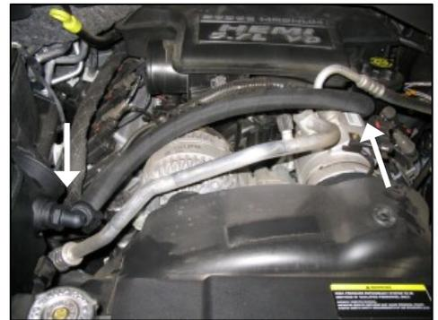
8. *5.7 Hemi engines only.* Using the supplied straight 3/4" hose, connect both ends to the nylon fitting and oil fill nipple as shown. Fasten both ends using the supplied nylon speed clamps. Adjust the nylon fitting downward to clear the factory intake tube assembly.
