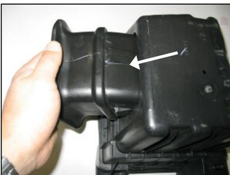
3. Using a 13mm socket, remove air box base from engine compartment. Using a flat blade screwdriver, carefully unsnap the box inlet from the base and remove it. Reinstall the factory base in the engine compartment with out the inlet.
