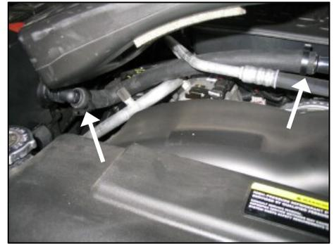
7. *4.7L engines only.* Using supplied pre-formed 3/4" hose, connect the nylon fitting to the remaining plastic factory hose as shown. Fasten both ends of the hose using the supplied nylon speed clamps. Adjust the fitting downward to clear the factory intake tube assembly.
