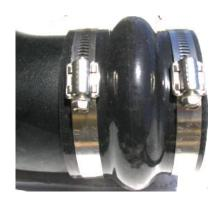
13. Install the black hump hose on the long end of the Airaid tube using two of the #56 hose clamps provided. Leave loose for final assembly.
