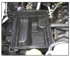
Unclip & remove the factory air box lid and factory air filter.
