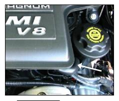
4. 2003 Models: Disconnect & remove the crankcase vent hose from the front of the factory resonator.
