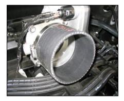
14. Slide the black coupler onto the throttle body and secure using a #56 hose clamp provided & install the 2<sup>nd</sup> #56 hose clamp on the other end of the coupler, leave loose for final assembly.
