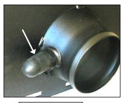
10. 2003 Models Only: Slip the black rubber cap over the nipple on the Cool Air Dam and secure using the #19 black speed clamp provided.
