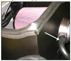
11. 2004-05 Models Only: Mount factory breather hose to the nipple on the Cool Air Dam and secure using the #24 black speed clamp provided.
