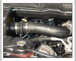
15. Slide the Airaid tube with hump hose into the Airaid Cool Air Dam first, and then slide the other end into the throttle body coupler. (*Note: The Airaid tube should be flush against throttle body*
