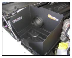
**8.** Position the Airaid Cool Air Dam in place of the original air box lid. Snap in place.
