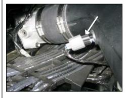
**16.** Re-connect air temperature sensor connector.
