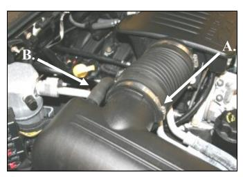
**2.** A.) Loosen the hose clamp on the factory airbox lid. B.) Disconnect the breather hose from the factory airbox lid.
