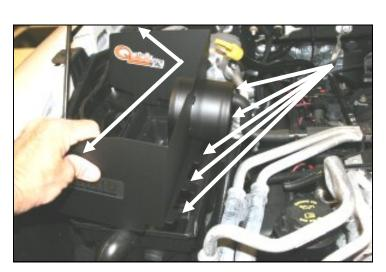
**5.** Slip the five tabs of the Quick fit panel (#2) through the slots on the airbox base. Adjust the panel for fit, then re-latch two of the factory clips onto the panel.
