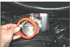
**3.** Remove the factory seal from the throttle body.
