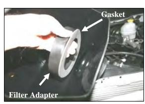
**8.** Install the adapter gasket (#25) and filter adapter (#6) into the **CAD** using three 1/4-20 x 5/8" bolts (#8) and flat washers (#9) as shown. *Refer to the line drawing above for reference.*
