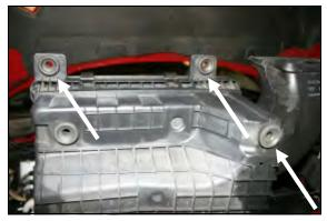
**6.** Remove and save three grommets from the bottom of the factory airbox. They will be reused in step #7.
