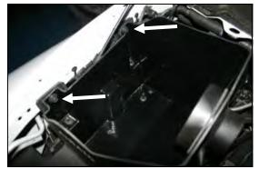
**10.** Install the **CAD** into the vehicle aligning the grommets over the locating pins. Reinstall the two factory bolts into the fender that were removed in step #9.
