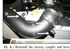
12. A.) Reinstall the factory coupler and hose clamps on to the Airaid intake tube (#2). Tighten the hose clamp on the tube. 2003-07 Models; B.) Install the supplied grommet (#11) into the hole in the Airaid tube, and then carefully push the factory air temperature sensor into the grommet. 2002 Models; Install the grommet plug (#10) in place of the grommet.
