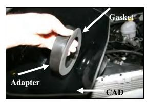
**6.** Install the filter gasket (#21) and filter adapter (#5) onto the Airaid Cool Air Dam (#3) as shown using three 1/4" x 5/8" bolts (#7), and 1/4" flat washers (#8). Refer to the line drawing above for reference.
