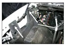
**9.** Remove the two bolts that secure the airbox mounting bracket to the inner fender. They will be reinstalled in step #10.
