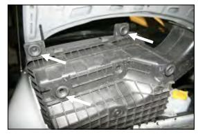
**3.** Turn the factory air box over and remove **3** of the 4 grommets. They will be reinstalled in the Airaid Cool Air Dam in step #8.
