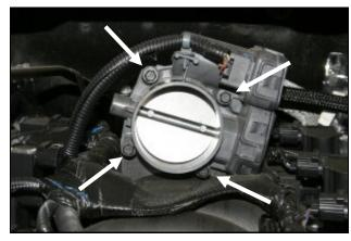
2. Remove the four bolts that secure the throttlebody to the intake manifold. Remove the throttlebody from the intake manifold and set it aside. (No need to disconnect the wiring harness.)
