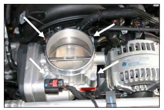
**4.** Reinstall the throttlebody on top of the Poweraid Spacer using the four bolts and washers that are supplied with the kit. Tighten the bolts evenly to the vehicle manufacturers specifications.
