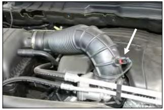
**5.** Reinstall the engine beauty cover and intake tube in the reverse order that they were removed. Make sure to reconnect the temperature sensor. **Re-connect the negative battery cable!**
