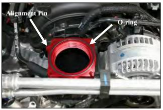
**3.** Install the supplied o-ring into the groove on the Poweraid Spacer. Next install the spacer onto the intake manifold with the o-ring facing up, making sure that the alignment pin holes are located over the alignment pins.
