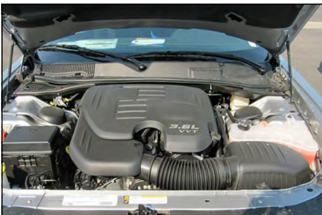
5. Reinstall the intake tube and engine cover in the reverse order that they were removed. Make sure to reconnect the temperature sensor.
