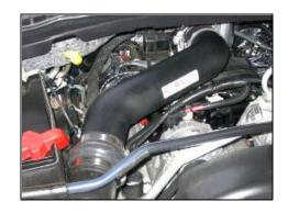
**9.** Check for any foreign objects or debris it the intake path & install Airaid MIT assembly on engine. (Note: Leave hose clamps loose until final assembly)
