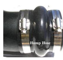
**8.** Install the hump hose and coupler provided onto the Airaid MIT with the supplied hose clamps. The straight coupler is positioned on the throttle body end and the hump hose is positioned on the air filter end.
