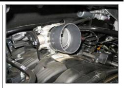
**7.** Install supplied reducer hose and #52 hose clamp onto the throttle body.
