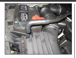
1. Disconnect the negative battery cable and remove the breather hose from the factory air box lid.
