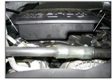
**5.** Loosen the two 10mm bolts mounting the factory air box to the intake manifold and remove from vehicle.
