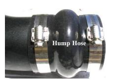
**8.** Slide hump hose on to straight end of Airaid intake tube with two #56 hose clamps. (*Note: Leave hose clamps loose until final assembly*).
