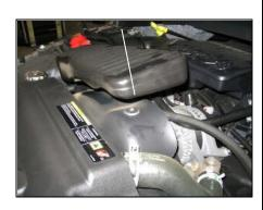
**3.** Unsnap the factory silencer box from the fan shroud and remove the factory tube assembly from the vehicle.
