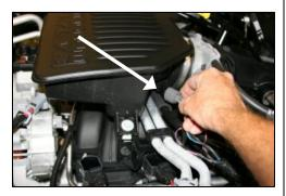
**2.** Disconnect the intake air temperature sensor by squeezing the tab on the connector.
