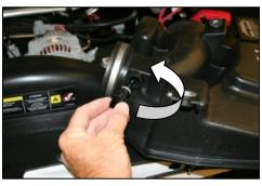
5. With the resonator turned over, carefully remove the air temp sensor by pushing in, and turning counter clockwise.
