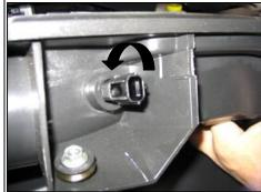
**5.** Remove air temperature sensor from housing by turning counter clockwise and pull.
