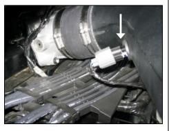
**10.** Reconnect electrical connector on factory air temperature sensor.
