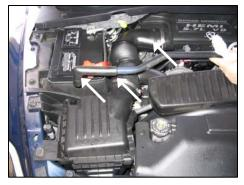
Disconnect negative battery cable. Remove valve cover breather hose from air box lid. Loosen hose clamps on both sides of factory intake tube.
