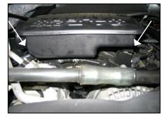
**5.** Loosen the two 10mm bolts mounting the factory air box to the intake manifold and remove from vehicle.
