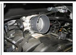
**7.** Install supplied reducer hose and #52 hose clamp onto the throttle body.
