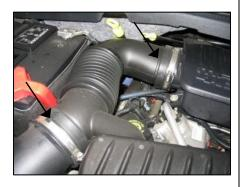
**2.** Loosen the two hose clamps on each end of the factory intake tube.
