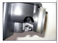
**6.** Turn the air temperature sensor \( \frac{1}{4} \) turn and remove from the air box. Retain sensor for later use.
