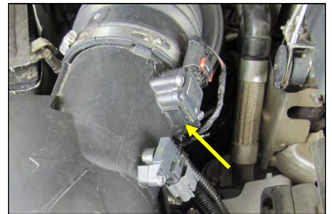
3. Gently pry the harness anchor out of its tab on the airbox and free the wire harness.
