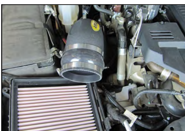
7. Slide the Hump Hose and clamps onto the Airaid Intake tube as shown.
