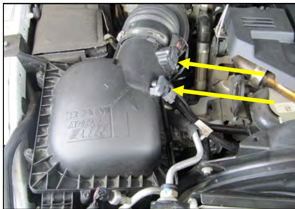
2. Disconnect both of the air sensors in the airbox top.
