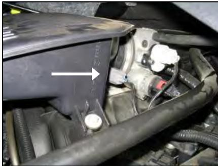
5. Disconnect the factory electrical connector from the factory air temperature sensor.
