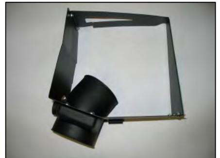
8. Using the supplied #6 screws, nuts and washers, assemble the two panels as shown above. Next, install the supplied air filter adapter using the supplied 1/4-20 bolts and washers.
