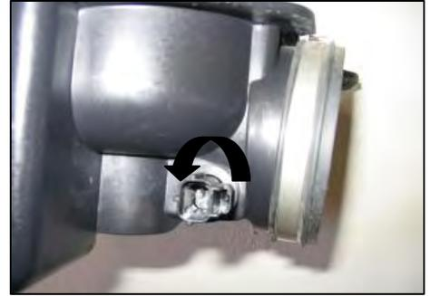
7. Turn the air temperature sensor 1/4 turn and remove from the air box. Retain sensor for later use.
