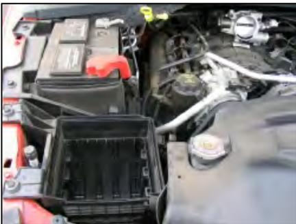
3. Unlatch the metal clips and remove the lid from air box base. Using a 13mm socket, remove the air box base from the engine compartment.
