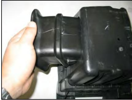
4. Using a flat blade screwdriver, carefully unplug the box inlet from the base and remove it. Reinstall the factory base in the engine compartment with out the inlet.
