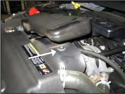
2. Unsnap the factory silencer box from the fan shroud and remove the factory tube assembly from the vehicle.
