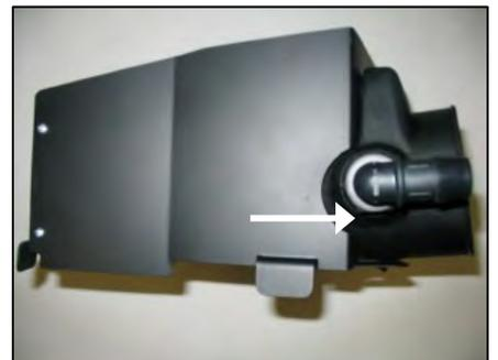
9. Install the supplied nylon fitting into the air filter adapter as shown.
