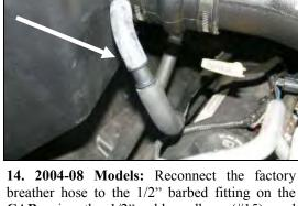
CAB using the 1/2" rubber elbow (#15), and 1/2"x 3/4" barbed fitting (#20) as shown.
