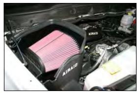
16. Install the Airaid Premium Filter (#1) onto the Airaid filter adapter, and tighten the hose clamp. Install the weather strip (#7) onto the top of the CAB, starting at the fender, and working your way towards the radiator.
