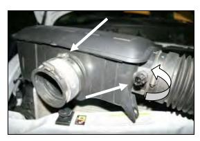
**5. 2002-07 Models** Loosen the factory hose clamp on the coupler and remove the coupler assembly from the resonator. **2003-12 Models:** Rotate the air temp sensor counterclockwise remove it from the resonator. These parts will be reinstalled on the Airaid intake tube in step #12.
