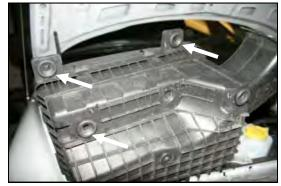
**3.** Turn the factory air box over and remove **3** of the 4 grommets. They will be reinstalled in the Airaid Cool Air Box in step #8.
