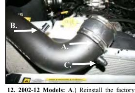
coupler and hose clamps on to the Airaid intake tube (#2). (2008 Models: use the supplied coupler (#5), and #48 hose clamps (#10). Tighten the hose clamp on the tube.
