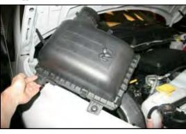
**2.** Slide the flexible intake tube off of the airbox lid and then lift the complete airbox straight up and out of the vehicle.
