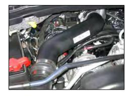
**9.** Check for any foreign objects or debris it the intake path & install Airaid MIT assembly on engine. (Note: Leave hose clamps loose until final assembly)
