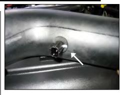
**7.** Install the supplied grommet and factory air temperature sensor into the Airaid MIT.
