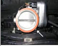
**6.** Remove factory orange seal from throttle body.
