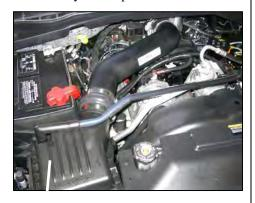
11. Adjust hose assembly for final position and tighten all four hose clamps. Reconnect valve cover breather hose to air box lid and replace oil fill cap.
