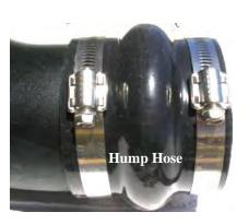
**8.** Install the hump hose and coupler provided onto the Airaid MIT with the supplied hose clamps. The straight coupler is positioned on the throttle body end and the hump hose is positioned on the air filter end.
