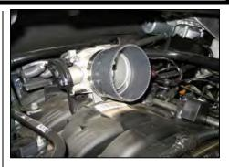
7. Install the reducer hose and a #52 hose clamp onto the throttle body. Install a #56 hose clamp onto the other side of the reducer.
