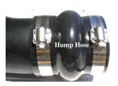
**8.** Slide the urethane hump hose onto straight end of Airaid intake tube with two #60 hose clamps. (*Note: Leave hose clamps loose until final assembly*).
