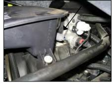
**4.** Disconnect the factory electrical connector from the factory air temperature sensor.
