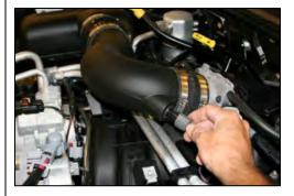
**9.** Install the MIT into the hump hose first, and then into the reducer. Adjust the MIT so that it's up against the throttle body, and then tighten all four hose clamps. Reconnect the air temp sensor.
