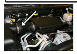
1. Disconnect negative battery cable. Loosen hose clamp on intake tube at the factory airbox end. For Jr. Kit, replace the factory air filter with the Airaid Premium Filter provided.
