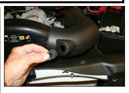
7. Install the grommet into the hole in the MIT as shown.
