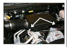
**3.** With the 10mm socket, remove 2 bolts from the base of the resonator.
