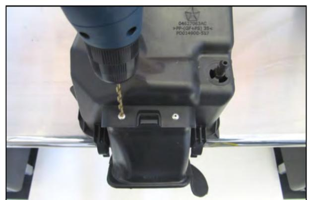
6. Drill out the rivet heads on the factory airbox and remove the air scoop.
