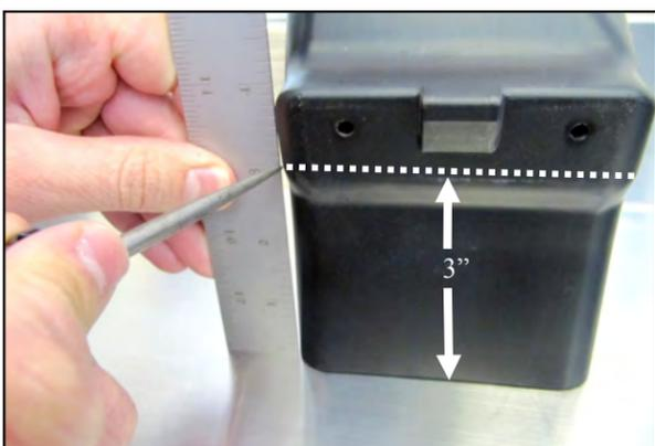
7. Set the factory air scoop on a workbench and mark all four corners at the three inch mark using a scratch awl. Using a straight edge and the awl, scribe a line connecting all four corners.
