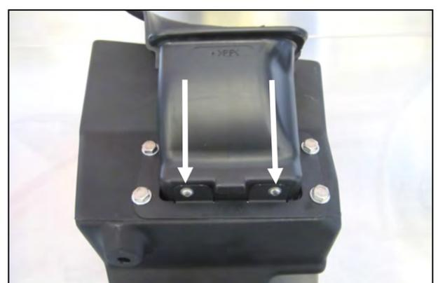
9. Insert the factory air scoop into the Cold Air Box and secure it using two 8-32 x 3/8" Button Head Bolts (#13), #8 Flat Washers (#14), and #8 Kep Nuts (#15).
