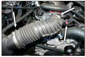
4. Reinstall the factory intake tube, and tighten the 2 hose clamps. Reconnect the wiring harness to the intake tube temperature sensor. Make sure you push down the red tab, and lock the harness.
