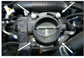
2. Using a 6 point 5/16" socket, remove the 4 bolts that hold the throttle body to the intake manifold.
