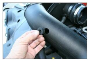
**11.** Install the supplied grommet into Airaid MIT as shown.
