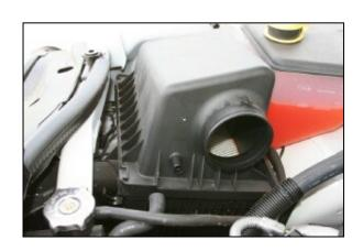
**8.** If you purchased an Airaid Jr. Kit, unhook the two clips and remove the factory air filter, and replace it with the Airaid Premium Filter supplied in the kit.
