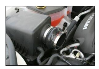
**9.** Reconnect the breather hose. Install the hump hose and two #60 hose clamps as shown. **Do not** tighten the clamps.
