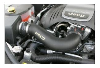
**13.** Install the MIT into the hump hose first, and then into the throttle body coupler. Adjust to fit, and tighten the hose clamps.
