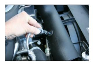
**12.** Carefully install the temperature sensor into the Airaid MIT as shown. Make sure it's pushed all the way in and the plug is connected to the wire harness.
