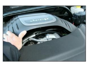
**14.** Re-install the engine cover by firmly pushing it back into the grommets.
