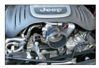
10. Install the coupler and two #60 hose clamps on the throttle body as shown. Do not tighten hose clamps. Fasten the factory breather hose to air conditioning line using the supplied zip tie.
