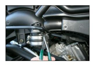
**5.** Carefully pull the intake towards you and rotate it so the bottom faces you, and cut the tie wrap that holds the breather tube, as shown
