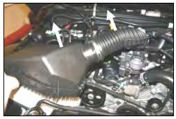
**4.** Remove the factory intake tube, and lid from the vehicle as an assembly.
