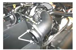
16. Install the Airaid Intake Tube into the hump hose first, and then rotate it down, and into the CAD. Install two 1/4" button head bolts (#7), and 1/4" flat washers (#8) thru the CAD, and into the inserts in the tube. Adjust for fit, and tighten both hose clamps, and bolts.
