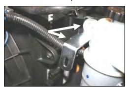
**10.** Insert the bolt, removed in step #8, thru the round hole in the provided L-bracket, and back into the radiator support. Leave the bolt slightly loose for now.
