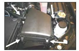
**3.** Unlatch the 4 metal clips that hold the factory air cleaner lid to the base. Next disconnect the breather hose that attaches to the rear of the air cleaner lid.
