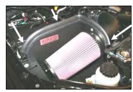
18. Install the Airaid Premium Filter (#1) onto the intake tube, and tighten the clamp. Next install the weatherstrip (#6) onto the top of the **CAD** as shown.
