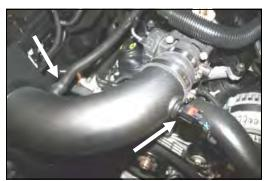
17. Very Carefully reinstall the temperature sensor removed in step #1, into the grommet in the Airaid Intake Tube. Reconnect the factory breather hose to the nipple on the intake tube.
