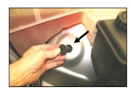
**9.** Slip the well nut (#22) into the hole in the inner fender.
