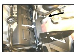
12. Install the rear support bracket (#6) from the **CAD** to the inner fender using three  $\frac{1}{4}$  - 20 x 1/2" button head bolts (#13),  $\frac{1}{4}$ " flat washers (#14), 1/4" serrated nuts (#15), and the 10mm factory nut removed in step #11.
