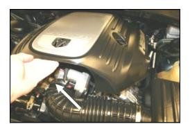
**1. Disconnect the negative battery cable.** *If you are working on a 5.7L, first remove the engine beauty cover by lifting it up off of the grommets.* Next, loosen the hose clamp that holds the factory intake tube to the throttle body.
