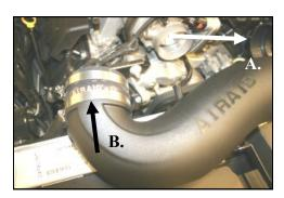
13. A. Install the urethane hump hose (#7) onto the filter adapter using two #72 hose clamps (#20), (*Leave loose for now*).
