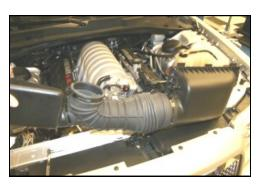
**5.** Remove the factory intake hose and lid assembly from the vehicle. Remove the factory air filter.
