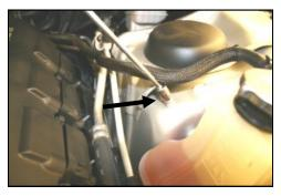
**11.** Remove the 10mm nut from the stud on the driver's side inner fender and save it for the next step.
