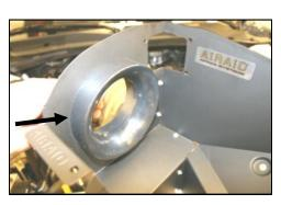
**8.** Next, install the filter adapter (#5) using three  $\frac{1}{4}$  - 20 x 1/2" button head bolts (#13), and  $\frac{1}{4}$  flat washers (#14).
