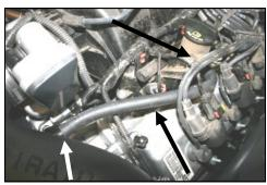
**17.** If you are working on a 6.1L, skip to step #18. If you are working on a 5.7L, install the breather hose (#9) from the valve cover to the Airaid Intake Tube as shown. Re-install the beauty cover onto the engine
