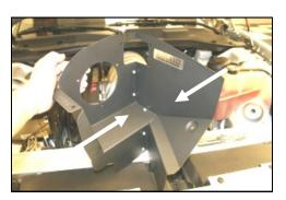
7. Assemble the two Cool Air Dam (CAD) panels (#2, #3) using five 6-32 x 5/16" screws (#16), #6 flat washers (#17), and 6-32 keps nuts (#18).
