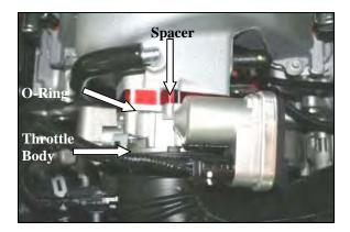
3. Install the O-Ring (#2) into the groove on the Poweraid Spacer (#1). Install the spacer between the intake manifold, and the throttle body with the O-Ring facing the throttle body. Insert four 6mm x 60mm Hex Bolts (#3), and 6mm Flat Washers (#4) through the throttle body, Poweraid Spacer, and into the intake manifold. Using a 10mm socket, tighten all 4 throttle body bolts evenly, to the manufacturer's specifications. **Do Not Over Tighten The Bolts!**
