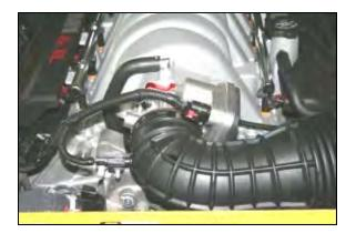
4. Reinstall the factory intake tube, and tighten the hose clamp. Reconnect the Air temperature sensor and throttle body motor. <u>Re-connect the negative battery cable!</u>
