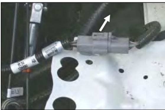
8. **4.2L Engine Only:** Using a flat blade screwdriver, carefully pry the MAF sensor wiring harness connector from the holes in the airbox mounting plate (*do not disconnect it*). Move the harness towards the firewall to allow room for the CAD to mount.
