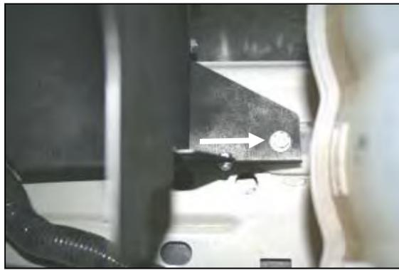
**11.** Align the hole in the CAD with the hole in the factory coolant reservoir mount. Insert one M6-1x25 hex bolt (#15) and 1/4" flat washer (#10) through the hole in the CAD, through the coolant reservoir mount, and into the speed nut below.
