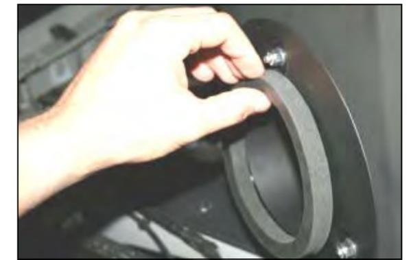
6. Install the supplied gasket (#13) onto the filter adapter.
