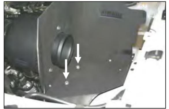
**12.** Insert two 1/4-20 x 7/8" bolts (#9) and 1/4" flat washers (#10) through the holes in the CAD and thru the grommets. On the underside of the factory airbox mounting plate, align the long/narrow bracket (#16), two 1/4" flat washers (#10), and two 1/4-20 nuts (#12) with the 1/4-20 x 7/8" bolts. Tighten the assembly securely.
