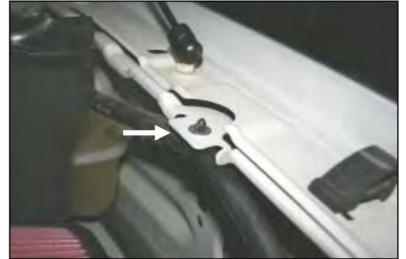
**15.** Slip the black plastic hose mount (#17) over the radiator overflow hose. Next, place one 1/4" flat washer (#10) over the hole on the inner drivers side fender. Slide the hose mount prongs thru the fender and thru the washer to secure the overflow hose.
