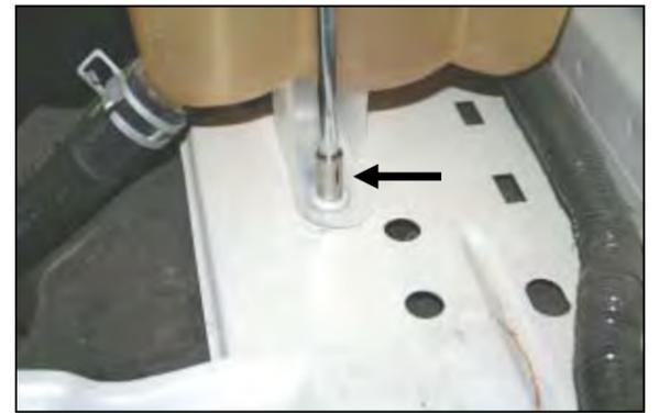
3. Using a 5/16" socket, ratchet and extension, remove one bolt from the factory coolant reservoir mount.
