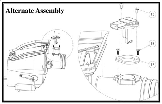
**Special Note:** Due to multiple factory mass air sensor calibrations, some vehicles may require the installation of the mass air flow sensor calibration plate and hardware as shown above. It may not be necessary to go to a dealer if your vehicle triggers a M.I.L. (Check Engine Light). Install the alternate assembly, or call Airaid for technical assistance.
