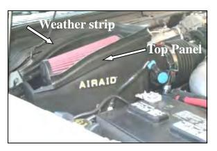
**10.** Install the Airaid Premium Filter (#1) onto the filter adapter, and tighten the hose clamp. Next install the Top Panel (#3) onto the top of the Cool Air Box using six 8-32x3/8" button head bolts (#10), and #8 flat washers (#11). Install the weather strip (#5) onto the edge of the top panel as shown.
