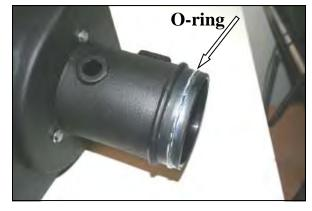
**6.** Install the O-ring (#14) into the groove on the Cool Air Box as shown. Apply a *light* coat of the supplied grease onto the O-ring.
