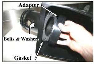
**4.** Install the adapter gasket (#13), and filter adapter (#4) into the Airaid Cool Air Box (#2) using three 1/4-20x5/8" hex bolts (#6), and 1/4" flat washers (#7).
