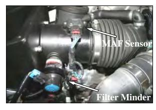
**9.** *A.*) Reinstall the factory grommet, and filter minder into the Cool Air Box, and then reconnect the filter minder wiring harness.
