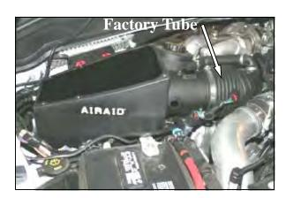
**7.** Apply a *light* coat of the supplied grease onto the inside of the factory tube. Install the Airaid Cool Air Box into the vehicle making sure it is seated correctly into the factory grommets, and the inlet is aligned with the factory hole in the fender. Slide the factory intake tube over the O-ring and then tighten the factory hose clamp.
