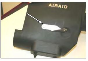
**5.** Install the bracket (#12) using one 1/4-20x5/8" hex bolt (#6), 1/4" flat washer (#7), and 1/4-20 serrated nut (#8) as shown. Just snug the bolt for now, it will need to be adjusted in step #8.
