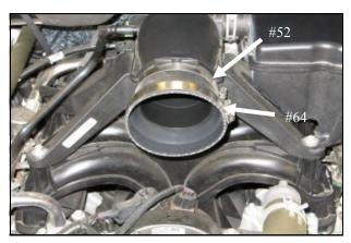
7. Install the Silicone Coupler (#6), one #64 Hose Clamp(#14), and the #52 Hose clamp (#13) onto the engine air inlet. Leave the clamps loose for now.
