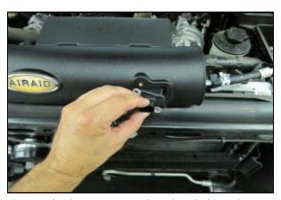
**8.** Transfer the **MAF** sensor into the Airaid Intake Tube (#2) and secure using two 8-32 x 1/2" button head screws (#11). **Do Not Use The Factory Torx Head Screws!**
