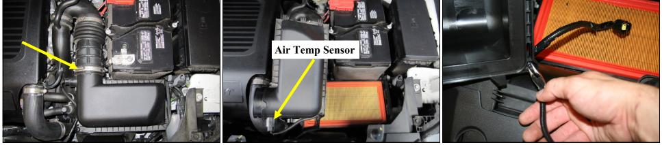
1. Disconnect the negative battery cable. Loosen the clamp on the air box side of the intake tube. 2. Unfasten the factory air box clips and separate the upper half of the air box from the intake assembly. Disconnect the air temperature sensor.
