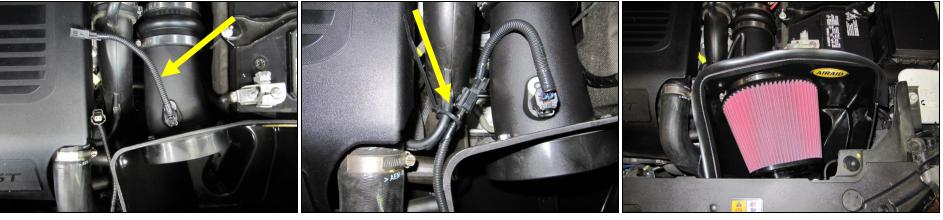
13. Connect the Wire Harness Extension to the air temperature sensor.
