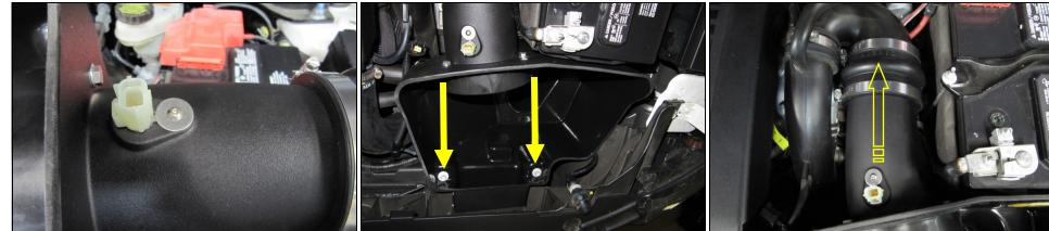
10. Transfer the factory Air Temperature Sensor into the Airaid Intake tube and align the sensor tab with the Groove in the tube. Secure the sensor to the tube using the 8-32 Button Head Bolt and the 3/4" washer.
