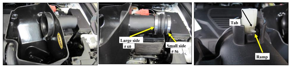
7. Install the Filter Adapter to the inside of the Cool Air 8. Install the Hump Hose, large side first onto the Intake Box, using the three 1/4"-20 hex head bolts and 1/4" flat tube. Loosely install the #56 Hose Clamp on the small washers as shown.
