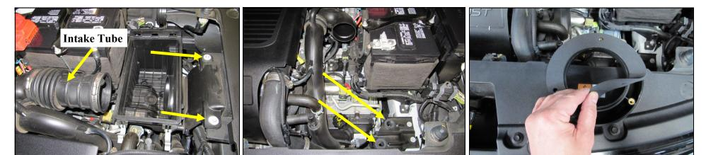
**4.** Using an 8mm socket, remove the two factory air box **5.** Remove the factory air box assembly from the vehicle. bolts and set aside. The will be reused in step 11. Loosen Be sure to retain the two air box mounting grommets. the second intake tube clamp and remove it from the vehicle
