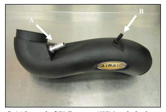
**8. A.)** Insert the 5/8" Grommet (#18) into the Intake tube as shown. Complete the tube assembly by inserting the 5/8 PCV Fitting (#16) into the Grommet. **B.)** Install the 3/8 " Hose Fitting (#20) into the threaded holt in the Intake Tube.
