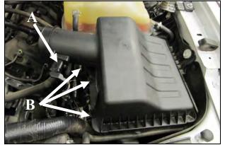
2. A.) Disconnect the Mass Air Flow (MAF) Sensor.
