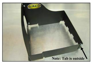
**4.** Assemble the two Quick Fit Panels (#4 & #5) as shown using four 6-32 screws (#12), flat washers (#13), and Kep Nuts (#14). The panel tabs are to be on the outside of the assembly.
