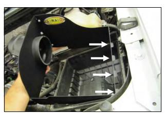
7. Install the assembly onto the lower half of the factory airbox. Slide the metal tabs into the airbox slots, and fasten the 3 airbox clips
