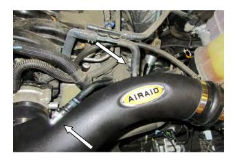
**12.** Reconnect the breather lines to the Airaid Intake Tube.
