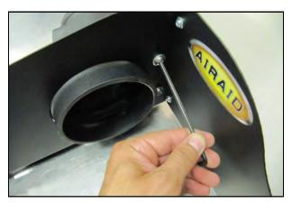
**5.** Install the Air Meter Tube (#2) onto the Panel Assembly and secure using the two 1/4-20 Button Head Bolts (9), and 1/4" Flat Washers (#10).
