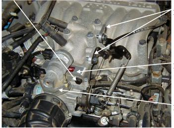
Ref. "C"- (2) 5/16-18" Linkage Plates (2) 8mm Flat Head Screws (2) 5/16-18" x 5/8" Bolts (2) 5/16" Flat Washers
