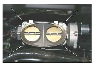
2. Using a 8mm socket, remove four bolts that hold the throttle body to the intake manifold.
