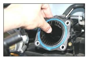
**3.** Remove the factory black plastic spacer that is located between the throttle body and the intake manifold.
