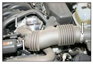
**1.** <u>Disconnect the negative battery cable!</u> Disconnect the crankcase breather hose from the engine air intake tube by pushing on the green tab, and removing the hose from the nipple. Loosen the hose clamp that secures the intake tube to the throttle body, and the one that secures the intake tube to the airbox lid. Remove the intake tube and set aside for now.
