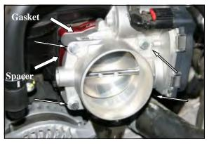
**3.** Insert the four 6mm x 75mm bolts (#3) with washers (#4) thru the throttlebody, one gasket (#2), and thru the Poweraid Spacer (#1), and into the intake manifold. Tighten all four throttle body bolts evenly, to the manufacturer's specifications. <u>Do Not Over</u> <u>Tighten The Bolts!</u>
