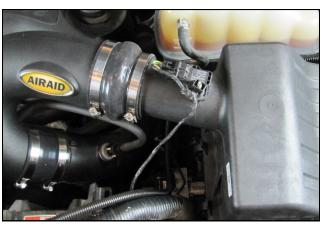
9. Reconnect the air meter or Map sensor and tighten all Clamps.
