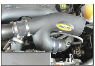
**4.** On late model vehicles, Install the  $1/4^{\prime\prime}$  Plug into the Airaid Intake Tube as shown. On 2011 models with the vacuum line in the intake, in-
