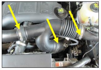
1. Disconnect The Negative Battery Terminal. Loosen the 3 clamps on the factory intake tube and remove it from the vehicle. NOTE: 2011 models will have a vacuum line attached to
