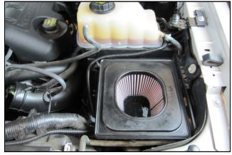
3. If installing an Airaid Jr. kit, replace the factory air filter with the Airaid Premium Filter at this time.
