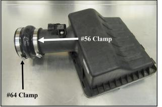
7. Slide the Hump Hose and the two remaining Clamps onto the OEM air box lid as shown.
